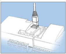
The controller must be switched on first and the LED "Status" must flash before the Service Tool programme is started.
