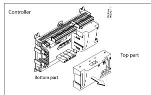
The controller is the cornerstone of the regulation. The module has inputs and outputs capable of handling small systems.
