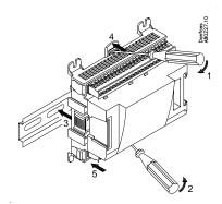
When the two snap catches for the DIN rail mounting are in the open position, the module can be pushed into place on the DIN rail – regardless of where the module is on the row.
