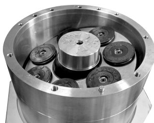
19. Place pistons in retainer plate and cylinder barrel, When pistons are placed, tilt retainer plate for easier placement of swash plate. If swash plate has been disassembled from mounting flange, see page 11 for assembly of swash plate.
