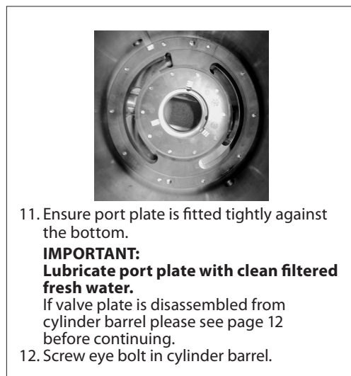
9. Place pump vertically. Place 10.5 mm pins in port flange. 10. Position port plate by using the two pins. Do not use force for this operation.
