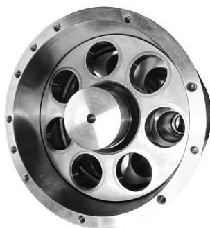
17. Place retainer plate in cylinder barrel. Note: (Remember to lubricate the retainer plate and cylinder bushings with clean filtered water).
