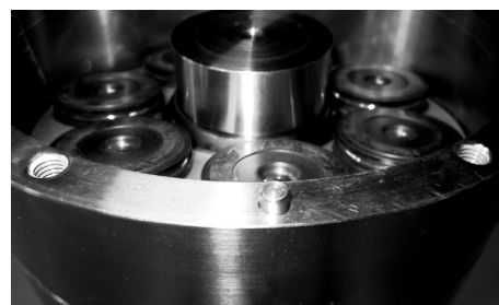
20. Place the guide pin in the housing. 21. Lubricate piston shoes and swash plate with clean filtered water. 22. Mount assembled swash plate, using the guide pin.
