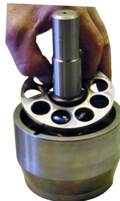
14. Remove the retaining plate.
