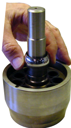
15.Remove the retaining ball.
