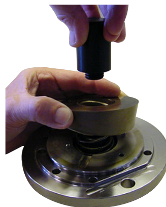
18. Press the swash plate against the flange and screw the tools together.
