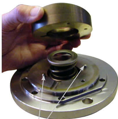
17. Mount the swash plate on the front flange using the pins as guide.
