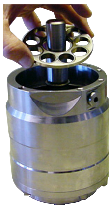
11. Mount the retaining plate (smallest centre diameter pointing upwards).
