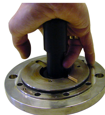
14. Mount the ceramic ring by pressing the tool as far down in the front flange as possible.
