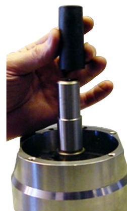
22. Mount the tool over the shaft.
