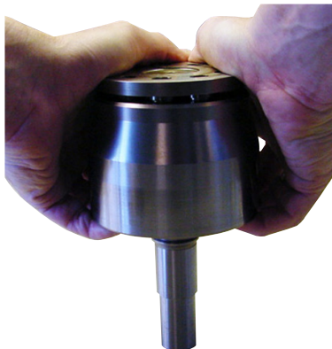
7. Press the thrust plate into the cylinder barrel using a table or the like as support.
