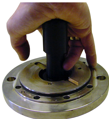
13. Mount the ceramic ring by pressing the tool as far down in the front flange as possible.
