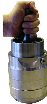
8. Mount the cylinder barrel in the housing.
