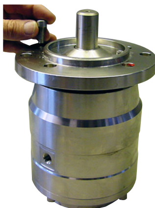
24. Mount the screws in the front flange.
