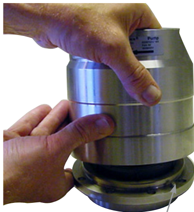
5. Mount the housing using the pin as guide.
