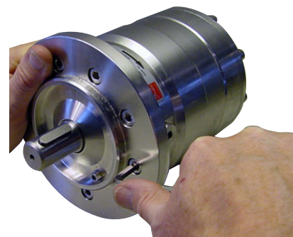
25. Tighten the screws to a torque of 30 Nm and mount the parallel key on the shaft.
