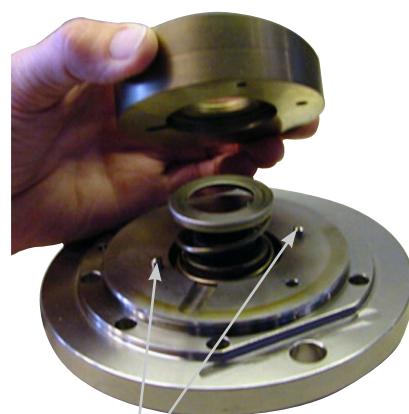
16. Mount the swash plate on the front flange using the pins as guide.
