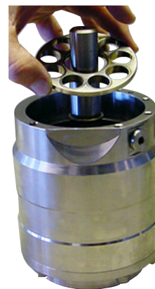
10. Mount the retaining plate (smallest centre diameter pointing upwards).
