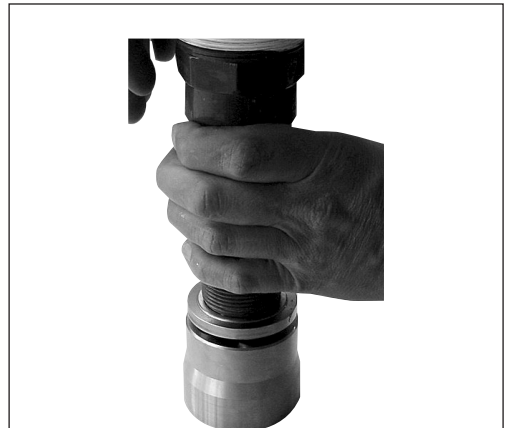
6. Press the valve plate into the cylinder barrel using a piece of plastic.
