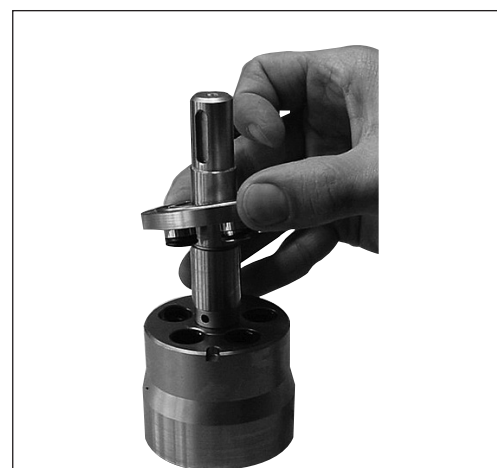
14. Remove the valve plate.
