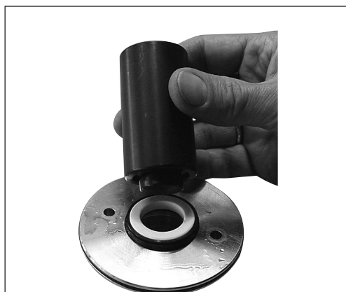
22. Wet the shaft seal with water and mount it in the front cover. Ensure that it is pressed to the bottom.
