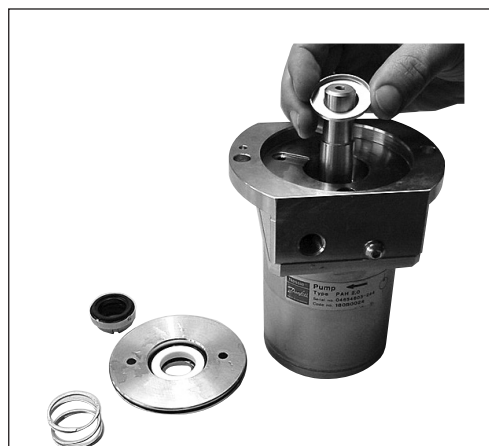
23. Mount the washer with the edge pointing upwards.
