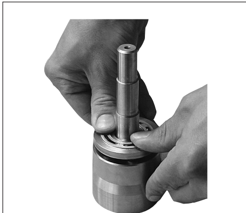
5. Mount the valve plate with seals on the cylinder barrel.
