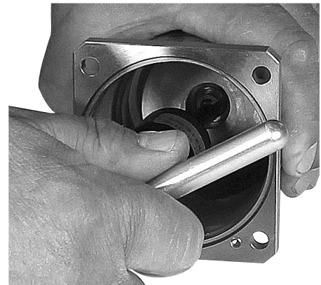
17. Tighten to a torque of 10 \pm 1 Nm.
