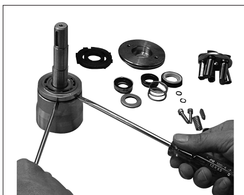
13. Loosen the valve plate using two screwdrivers. Place one of the screwdrivers in the slot of the valve plate.
