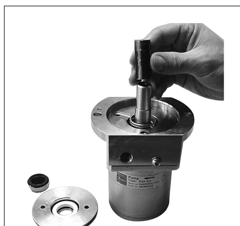
25. Fit the hollow bush onto the shaft.
