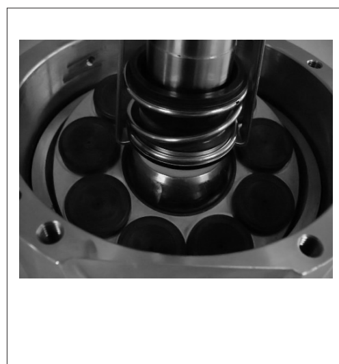
5. Carefully remove the shaft seal assembly using the shaft-seal extractor supplied. The extractor must fit underneath the shaft seal.
