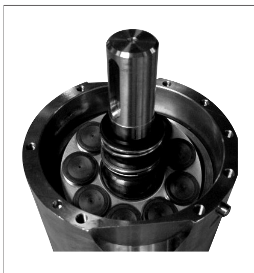
12. Remove the old O-ring and fit the new O-ring on the adapter.
