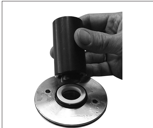
19. Wet the shaft seal with water and mount it in the front cover. Ensure that it is pressed to the bottom.
