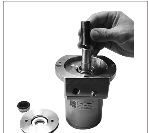
22. Fit the hollow bush onto the shaft.
