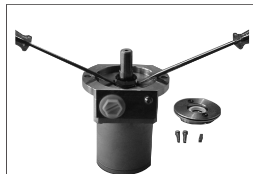
4. Remove the shaft seal using two screwdrivers. Caution: Avoid scratching the sealing surface on the shaft.
