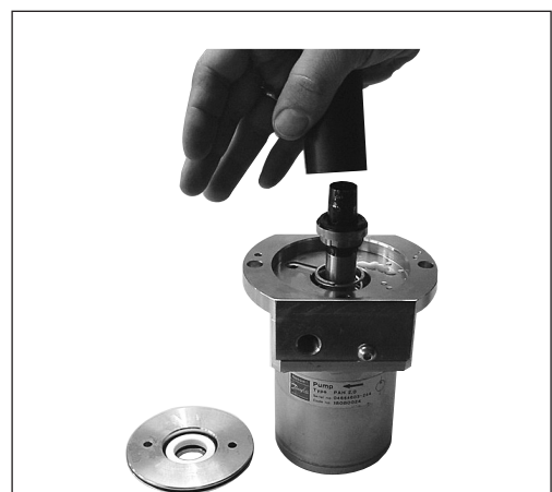
24. Use the shaft seal tool when pressing the shaft seal downwards.
