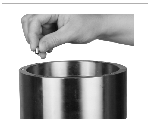
9. Mount 1 guide pin inside the housing on the back side of the port plate.
