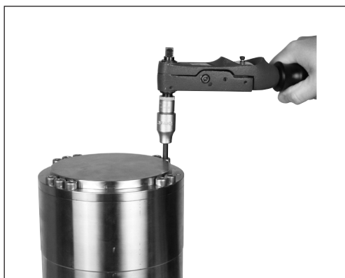
31. Tighten 10 screws to 30Nm.
