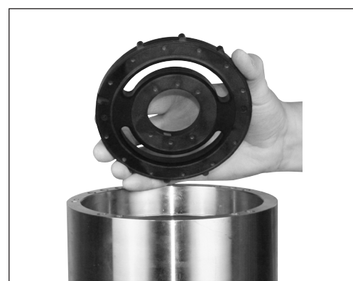
10. Mount port plate. Be aware of orientation/guide pin.
