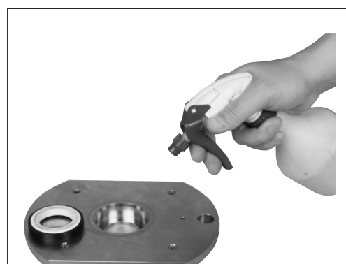
34. Spray shaft sealing with water before mounting.
