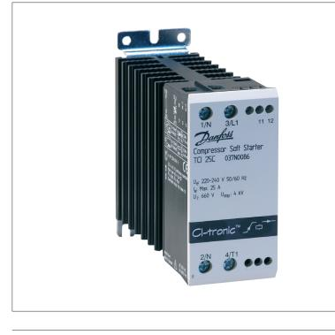
The TCI 25C soft starter is designed for soft starting of single-phase compressors. During start the TCI 25C will gradually ramp-up the motor voltage to full line voltage thus reducing the starting current peak.
