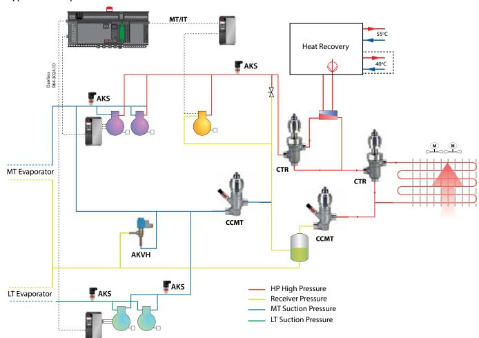
In CO<sub>2</sub> systems, the higher pressure and temperature make it possible to recover heat for tap water and heating. The excess heat is removed using a gas cooler.
