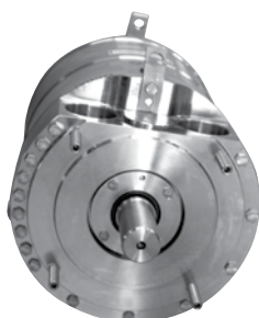
23. Screw in the rest of the bolts and cross tighten all screws to a torque according to exploded view.
