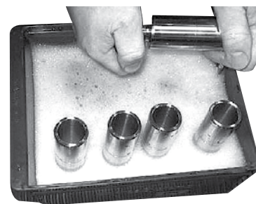
17. Place retainer plate in cylinder barrel. Note: If pistons are replaced, place new pistons in clean filtered water for a couple of minutes. Exercise piston shoes to make them "run" smoother.
