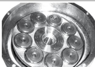
19. Place pistons in retainer plate and cylinder barrel. When pistons are placed, tilt retainer plate for easier placement of swash plate. If swash plate has been disassembled from mounting flange, see page 10 for assembly of swash plate. 20. Lubricate piston shoes and swash plate with clean filtered water. Remember to place the pins in housing. 21. Place the pins in the housing.
