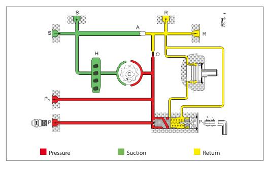
From the suction inlet (S) oil is drawn through the gear set, where the pressure is increased. By means of the piston and the spring in the pressure regulator the pressure is kept constant at the value set on adjustment screw (P1).
