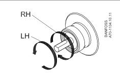
Note! Shaft rotation, location of nozzle outlet and other connections are seen from shaft end.
