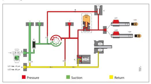
The LE pump is used with either an LE nozzle (System 1) or an LE preheater (System 2). Before burner start the preheater heats up the oil in the nozzle line. The expanding oil is prevented from dripping out of the nozzle because of the connection back to the suction side. The non return valve B inside the pump has an opening pressure of less than 2 bar whereas the LE valve in the nozzle opens at a pressure of 5±1 bar. (The valve in the preheater opens at min. 6 bar.)
