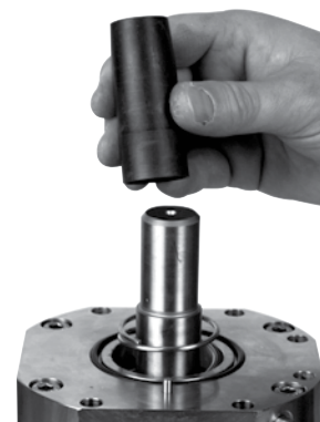
38. Mount special tool on shaft.
