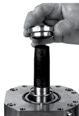
40. Mount sealing (smallest diameter pointing down).
