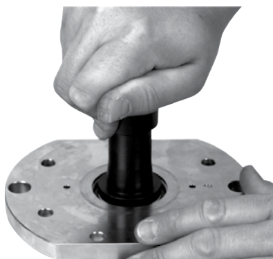
35. Use tool and press shaft sealing into place.
