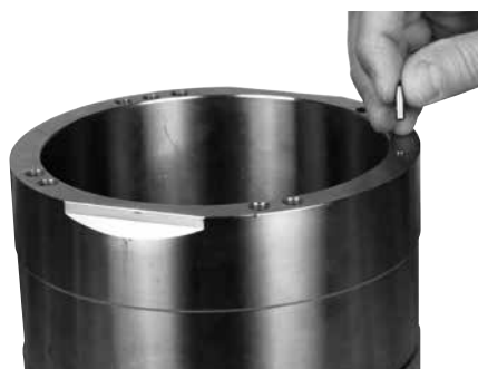
3. Mount 1 guide pin in housing.
