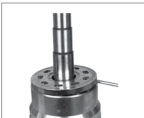
23. Loosen thrust plate from cylinder barrel.
