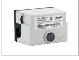
The microprocessor based control OBC 82.10 offers stable and precise timings independent of variations in supply voltage and ambient temperature. The control is undervoltage protected in accordance with EN 298:2012. In case of undervoltage the control will prevent the burner from starting and simultaneously show a flash code. Besides this, up to five other fault types can be read out as flash codes when the control is in lockout.
