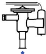
Angle flow (fixed orifice)
