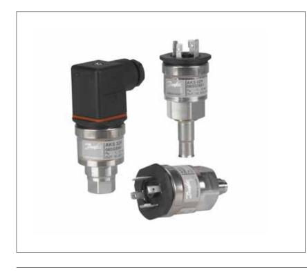
AKS 32R is a ratiometric pressure transmitter that converts the measured pressure to a linear output signal. The output signal is relative to the supply voltage meaning that the min. pressure output will be 10% of the actual supply voltage and the max. pressure output will be 90% of the actual supply voltage.
