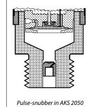
Cavitation, liquid hammer and pressure peaks may occur in liquid filled systems with changes in flow velocity, e.g. fast closing of a valve or pump starts and stops. The problem may occur on the inlet and outlet side, even at rather low operating pressures.
