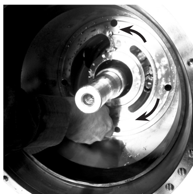
30. Remove the guide pins.
