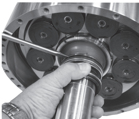
21. Remove the shaft seal by hand or using a screw driver between the washer and the shaft seal, if needed.
