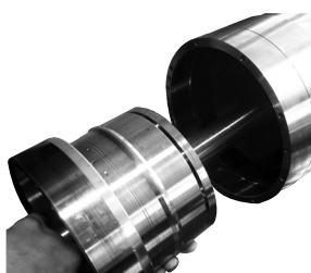
32. Carefully remove the cylinder barrel with shaft and valve plate. For more information on how to disassemble the valve plate assembly, please see the section "Disassembling and assembling of the valve plate".
