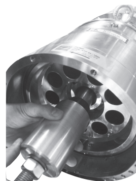
25. Remove the cone bushing. It was previously loosened in step 15 but if it is too tight using the cone bushing extractor again as described there.
