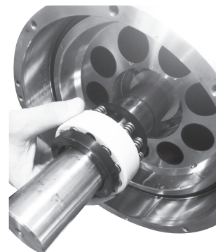
22. Remove pistons, retainer plate, retainer ball, distance washer, and spring package following the same steps described before for the end flange side (steps 10 to 13).
