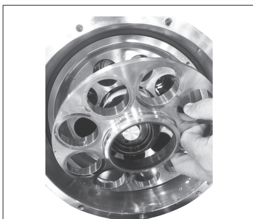
11. Remove the retainer plate.
