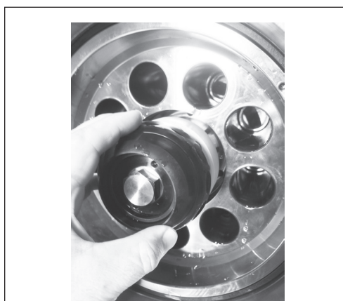
12. Remove the retainer ball.
