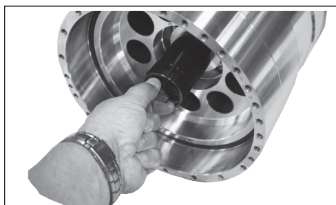
10. Remove by hand the pistons one by one. Be careful not to scratch the pistons. Tilt the retainer plate as needed for easy removal of pistons. When removing the last pistons, hold with one hand the retainer plate to make sure the retainer plate does not drop out. WARNING: Do not use any tools.
