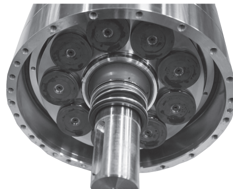
20. Remove the motor flange following the same steps described for the end flange (steps 2 to 9). Using the M8 x 140 mm is optional.
