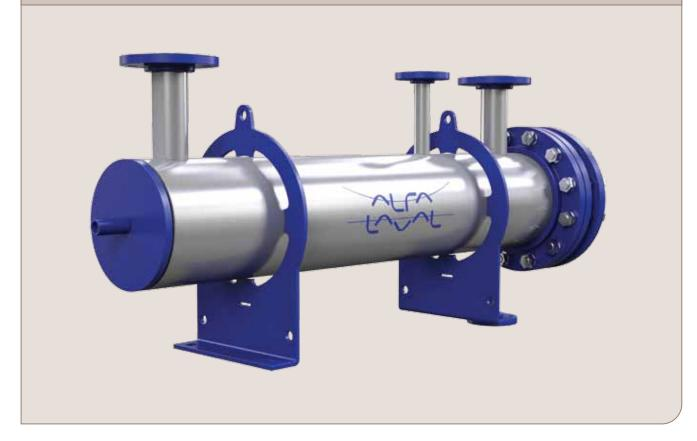
Aalborg MX is a compact shell and tube heat exchanger with U-tubes, ideal for heating or cooling of oil or water. The heat exchanger uses either steam or thermal oil as heating medium, and it uses either freshwater or seawater for cooling. Its heat load capacities range from 10 kW to approx. 5,000 kW, with design conditions (shell/tube) either up to 16/16 bar 160/204°C or 32/19 bar 195/212°C.
