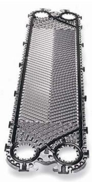
Standard: The most commonly used plate types for hygienic applications are the Alfa Laval M, T and Clip plate types. Their ideal press depth and relatively few contact points prolong operating times, while a unique distribution area ensures uniform flow over the entire plate surface. Clip plates on Alfa Laval FrontLine are specifically designed for heat-sensitive food products.
