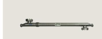
All tubes are connected in parallel and in counter-current flow to the service medium. The product tubes are corrugated. The service media shell is smooth.
