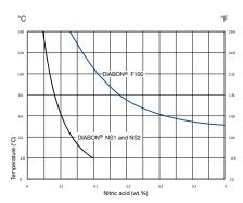
Compared with standard resin-impregnated graphite DIABON® F100 offers superior resistance in oxidating environments
