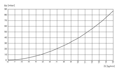
The diagram shows exemplarily the pressure loss characteristics when air flows through a flowmeter with 1/4" pipe connection. For determining the pressure loss with another gas it needs to calculate the air equivalent.
