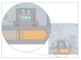
The measurement is based on the bypass principle. A laminar flow element in the main channel generates a small pressure drop. This drives a small flow, proportional to the main flow, through the bypass (sensor tube).
