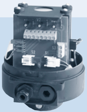
Control head without cover, PG9 screwed cable gland, multipole, 8-pole terminal strip for 24 V DC
