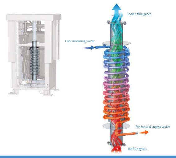
Heat is recovered from hot flue gases into the incoming supply water to save energy
