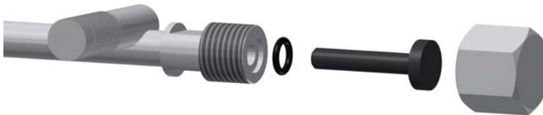
Fig. 22: Plugging pipe ends
