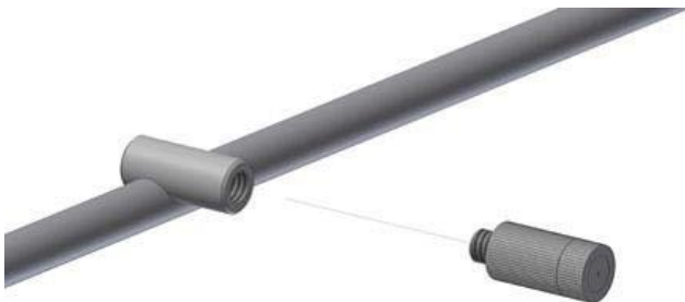
Fig. 20: Inserting the nozzles
