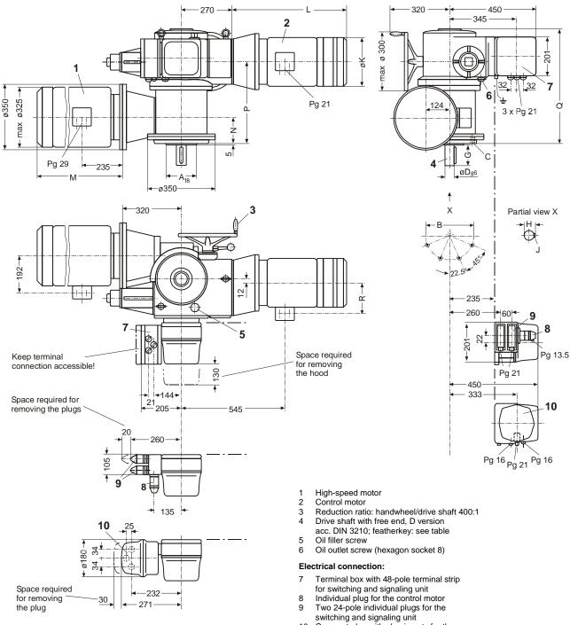
Compact plug with plug inserts for the control motor and the switching and signaling unit (2 x 24-pole)
