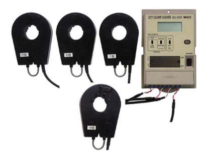
This is new measuring method for AC leakage current measurement of three phase 3 wire or three phase 4 wire power system. It is useful when working at the field where it is difficult to clamp the whole phase conductors.
