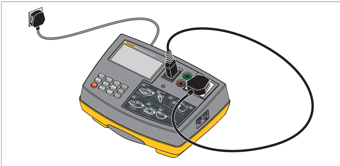
Figure 6. IEC-Lead Test Connections
