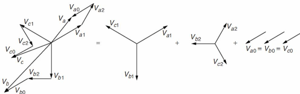
$$V_a = V_{a1} + V_{a2} + V_{a0}, V_b = V_{b1} + V_{b2} + V_{b0}, V_c = V_{c1} + V_{c2} + V_{c0}$$
