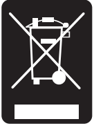
Fig. 1.4: Product labeling in accordance with EN 50419
