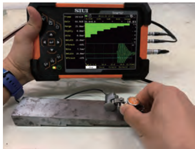
With PES-02D for encoded B-Scan
