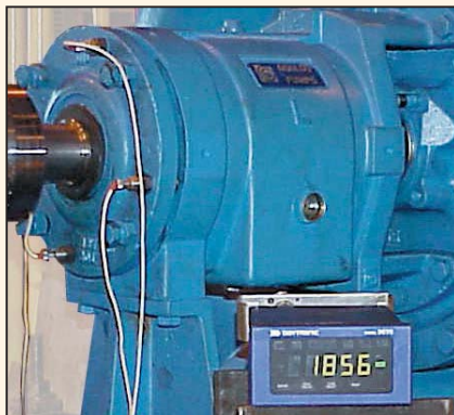
Bearing Load Measured on Test
