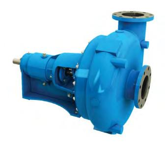
This Model HS Horizontal Hydro-Solids pump eliminates clogging problems encountered with conventional centrifugal pumps. The recessed impeller design handles large particle solids and fibrous/stringy materials. Any spherical solids that will enter the suction (up to 10") will pass through the discharge.
