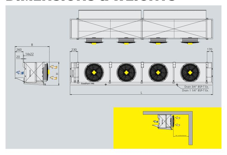
The Goedhart® VNS range of ceiling mounted aircoolers are specially designed for use in chill rooms, working with an air temperature of  $\pm$  0°C. The aircoolers are especially suitable for vegetable and fruit storage, working with a small  $\Delta$  T to prevent dehydration of the product. The height of the aircooler is low, so the maximum space in the chill room can be utilised.
