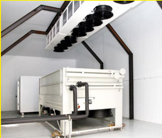
Unit under test in large calorimeter room
