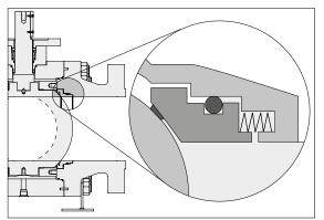
**Soft sealing seating ring (SO)** A seal ring made of plastic is used for sealing
