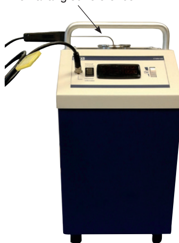
Temperature multi-function calibrator with an external angled reference
