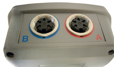
2 connection port for temperature probe inputs
