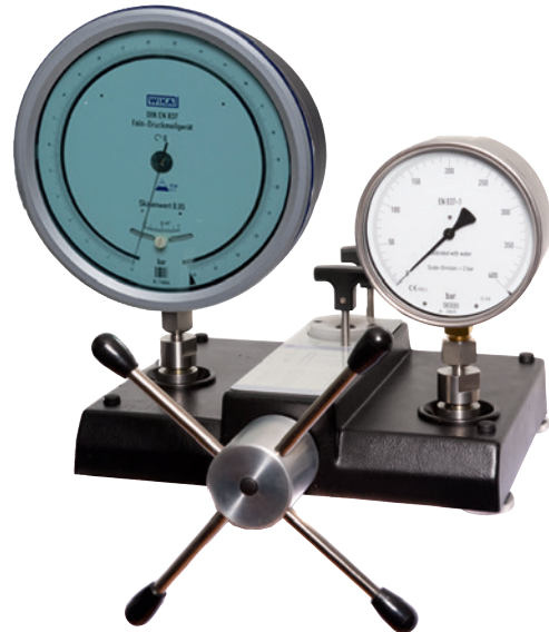
Calibration assembly CPP4000-X with test gauge as reference instrument and test item
