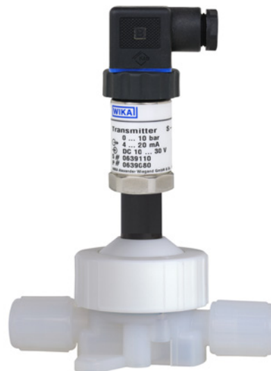
HYDRA-line Model HS, transducer 4 ... 20 mA, 2-wire system and in-line 1/2" flare process connection
