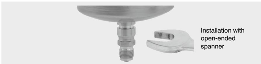
For parallel threads, use flat gaskets, lens-type sealing rings or WIKA profile sealings at the sealing face ①. With tapered threads (e.g. NPT threads), sealing is made in the threads ②, using a suitable sealing material (EN 837-2).
