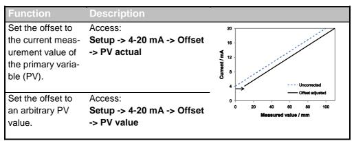
The standard value of the offset after reset to defaults is 40 mm above the lower sensor end.
