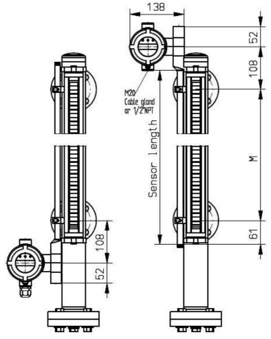
Level measurement on a magnetically operated liquid level gauge, sensor head downwards.
