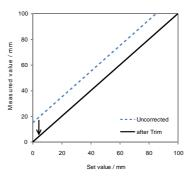
Remark: A trim can be applied to liquid level, interface, electronics
