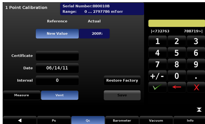
Figure 7.4.3.1a - 1 Point Calibration for Qc in [Vent] mode with [New Value] button pressed
