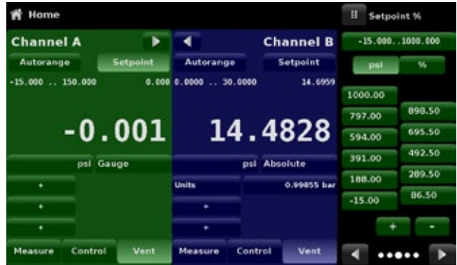
Figure 6.4.1.2.3-B - DUT Pressure Value Entry
