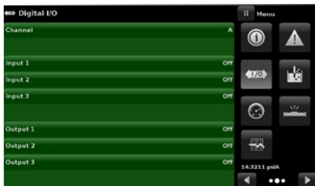
Figure 6.4.11-A - Digital I/O Application
