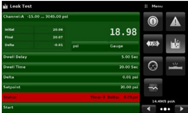
Figure 6.4.12-A - Leak test fail (left) & Leak test pass (right)
