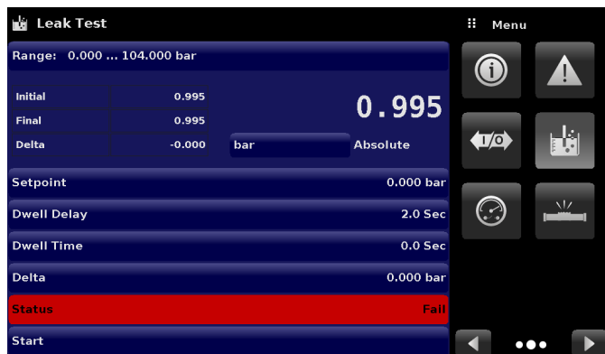
Figure 6.4.12-A Leak Test Fail (left) and Pass (right)
