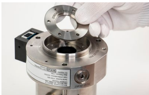
Figure 8.1.2.1.1-D Removing retaining ring
