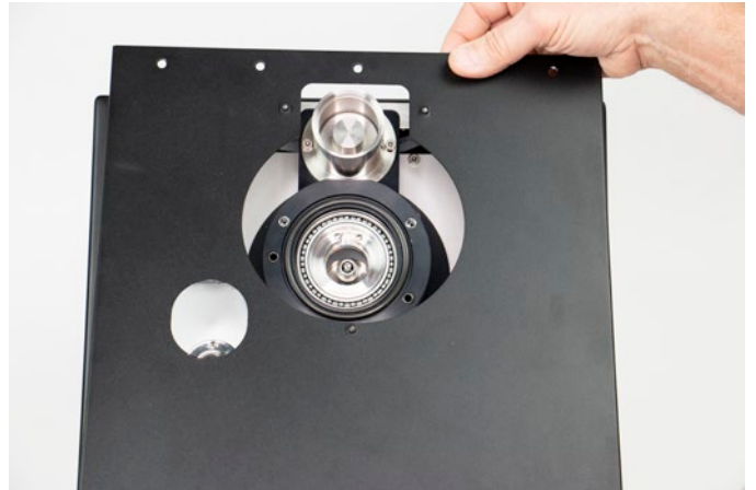
Figure 8.1.3.4-B Top Cover Removal
