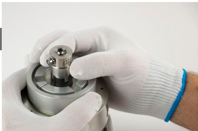
Figure 8.1.2.1.1-A Removing The Piston From Head
