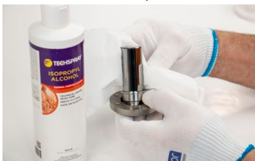
Figure 8.1.2.1.2-A Piston and cylinder cleaning
