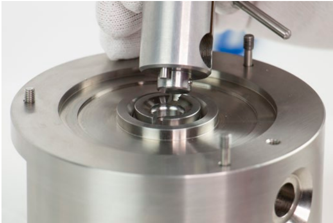
Figure 8.1.2.3.1-C Jam Nut Removal
