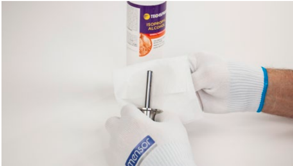
Figure 8.1.2.2.2-A Cleaning the piston and cylinder
