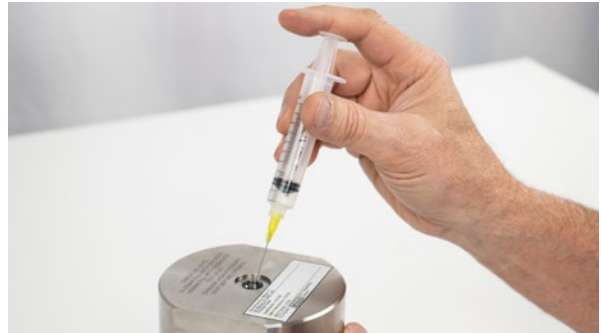
Figure 8.1.2.2.2-D Fill with oil
