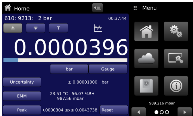
Figure 6.4.1.1-B Unstable Pressure Reading
