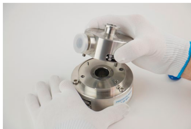
Figure 8.1.2.1.1-B Removing Top Cap
