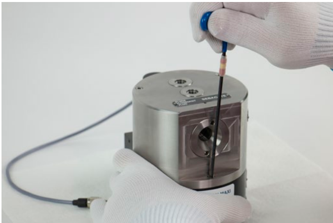
Figure 8.1.2.3.1-A Separating Measuring Head
