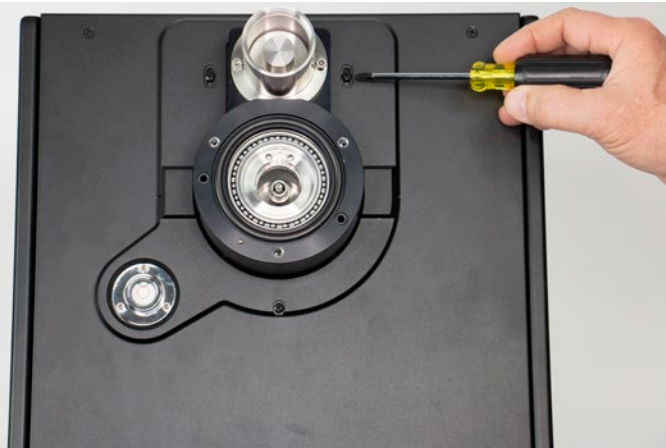
Figure 8.1.3.4-A Trim Plate Removal
