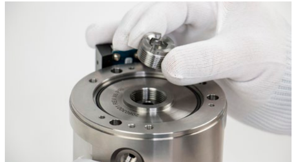
Figure 8.1.2.2.1-E Removing the cylinder jam nut
