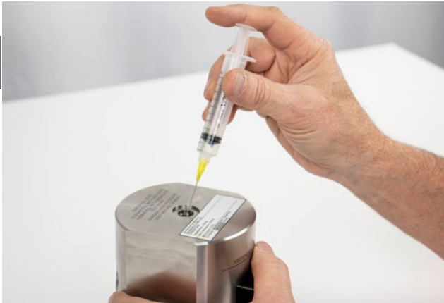
Figure 5.4.2-F Adding Oil to the Gauge Head
