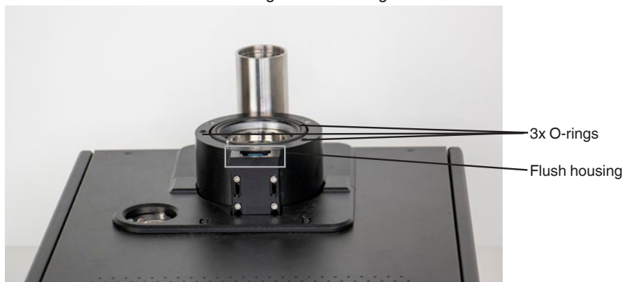
Fig 5.8.1-D Check O-rings and housing
