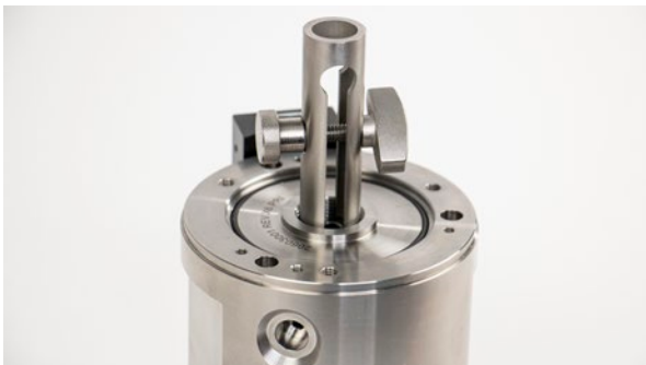
Figure 8.1.2.2.1-F Removing the cylinder
