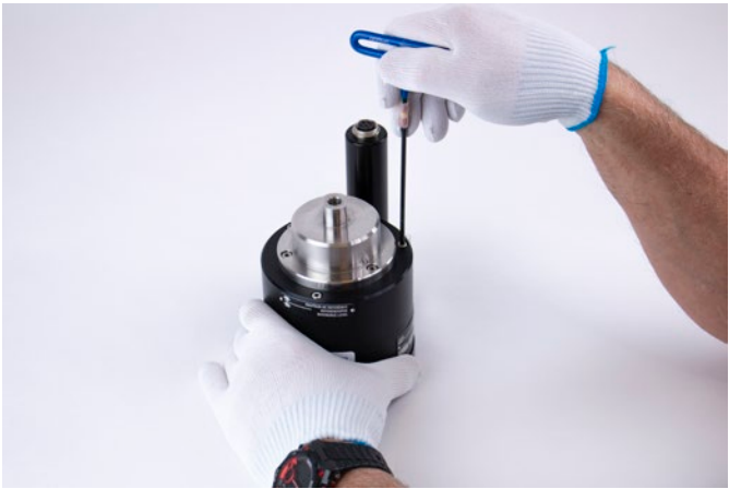
Figure 8.1.2.2.1-A Separating Measuring Head
