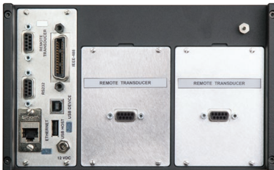
Figure 5.4 B - Two remote transducer interface connections installed
