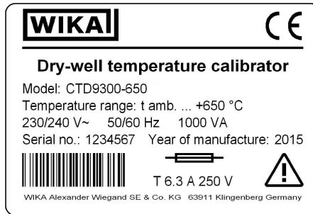
Fig. 38: Type label of a CTD9300
