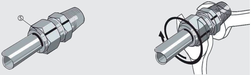
Securing the compression fitting
